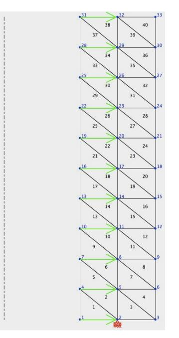
The model "Solid of Revolution" is used for volumetric parts. Volume must be generated by a surface that rotates about an axis.
