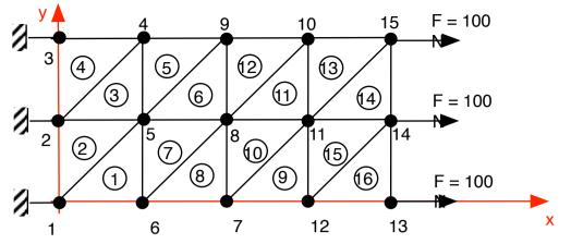
The model "plane deformations" is used for slice of structure where there is no deformation on z direction considered. For example: a section of a dam...
