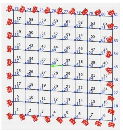
The model "Board flexion" is used for board with small thickness, witch perpendicular effort, and small deformations regarding to thickness. For exemple: Floor
